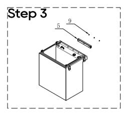
Fix the Wall Mounting Adapter to Cabinet with M4 Screws
