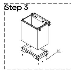
Fix the main cabinet to Floor Mounting Base with M6 screws.
