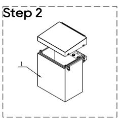
Untwist latches to remove the top cover of main cabinet
