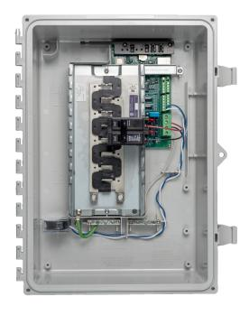
The Enphase IQ Combiner 3™ with Enphase IQ Envoy™ consolidates interconnection equipment into a single enclosure and streamlines PV and storage installations by providing a consistent, pre-wired solution for residential applications. It offers up to four 2-pole input circuits and Eaton BR series busbar assembly.
