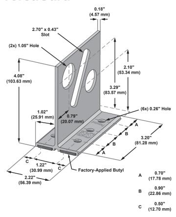
6 holes are provided for versatility. Some installations require only 2 fasteners. See the load table on the S-5! website and the installation instructions for more details.
