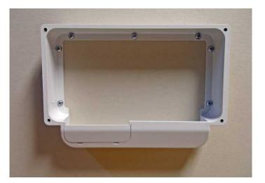
Make the wire connections to the terminal block inside the KID, replace the back plate and then assemble the KID to the wall mount adapter. Use the  $#10 \times \frac{3}{4}$ " Plastite screws provided to secure the KID to the wall mount adapter. Black units get black stainless steel screws and white units get natural stainless steel screws.
