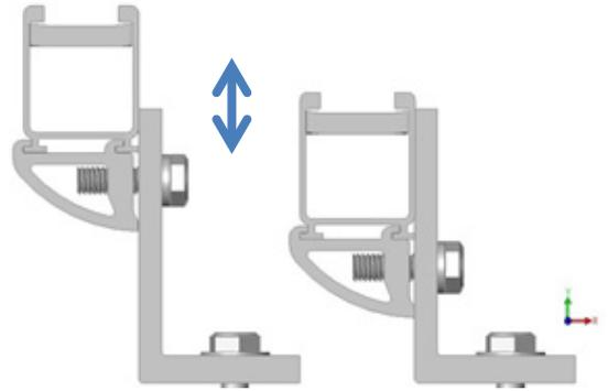
If there are multiple rows of rails in the array, use a string level or straight edge to help adjust the remaining rows to be level with the top and bottom rails. It is also possible to visually align rails in the middle of the array.
