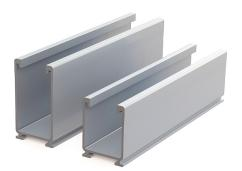
Two Rail Sizes in Mill Finish 2.3-inch rall for heavy loads and longer spans and 1.6-inch rail for low-profile mounting and areas with low snow load.
