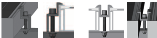
Figure2. SPV module installed with clamp fitting method
