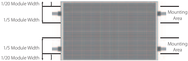
Figure3. Mechanical dimensions when modules installed at orientation with Clamp fitting method
