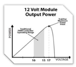
difference between the Vmp and the battery, the more "boost" current the battery will receive. The graph on the left illustrates the advantage of operating at the TrakStar MPPT.
