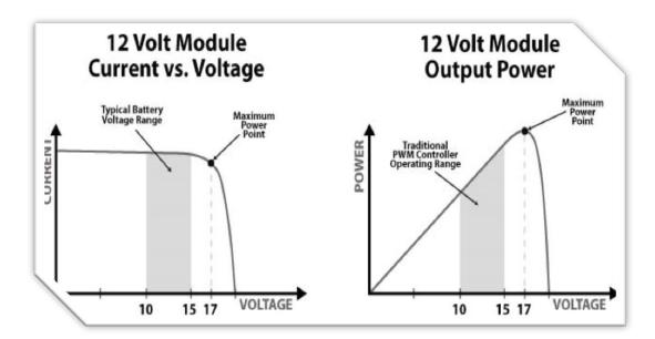
Because these traditional controllers rarely operate at the Vmp of the solar array, potential energy is being wasted that could otherwise be used to better charge the battery bank and maintain power for system loads. The greater the difference between battery voltage and the Vmp of the array, the more energy is wasted by a PWM controller during bulk charging.
