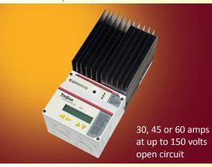
Morningstar's **TriStar MPPT** solar controller with TrakStar Technology™ is an advanced maximum power point tracking (MPPT) battery charger for off-grid photovoltaic (PV) systems up to 3kW. The controller provides the industry's highest peak efficiency of 99% and significantly less power loss compared to other MPPT controllers.
