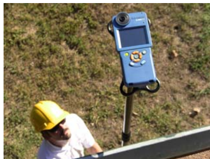
Figure 2-57. SunEye Extension Kit
