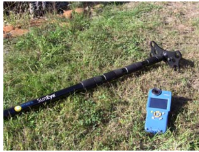
Figure 2-58. The SunEye Extension Kit
