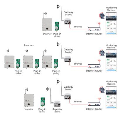
Scenario B: Adding additional ZigBee Plug-ins Part Number: SE-ZBSLV-B-S1-NA - 1x ZigBee Plug-in for connecting multiple inverters to the same ZigBee gateway
