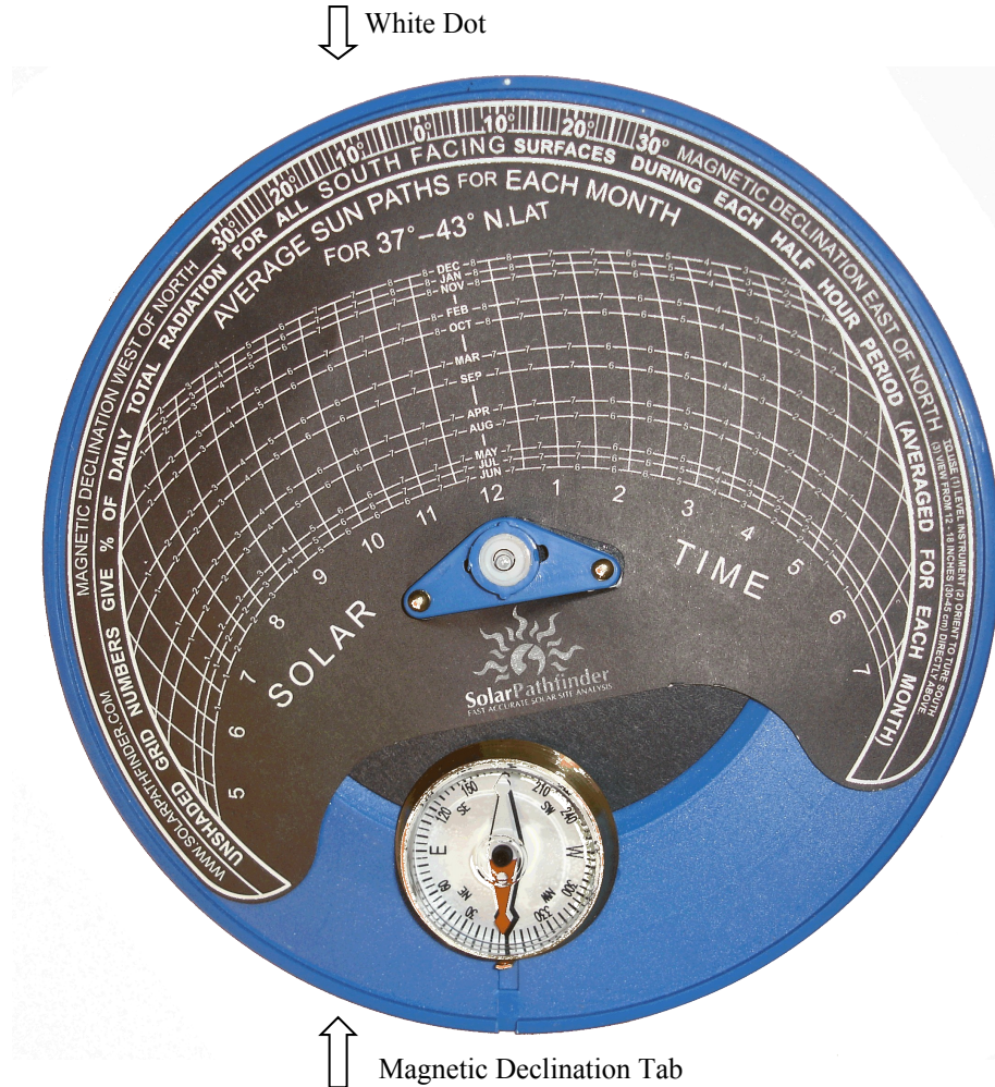
Figure 3 Magnetic Declination for 11 degrees east of north (+11 degrees)
