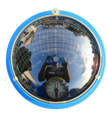
The Solar Pathfinder<sup>TM</sup> uses a highly polished, transparent, convex plastic dome to give a panoramic view of the entire site. All the trees, buildings or other obstacles to the sun are plainly visible as reflections on the surface of the dome. The sunpath diagram can be seen through the transparent dome at the same time.
