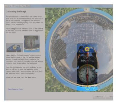
10. Calibrate the site picture by simply cropping it and aligning the level and declination settings directly on the picture you have taken.
