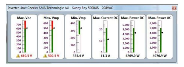
Green bars only are shown when the limits are not exceeded, and the arrow on the right of each value shows the calculated value. If limits are exceeded, a red bar is shown in addition to the yellow caution triangle, as shown above for DC Power and AC Power.
