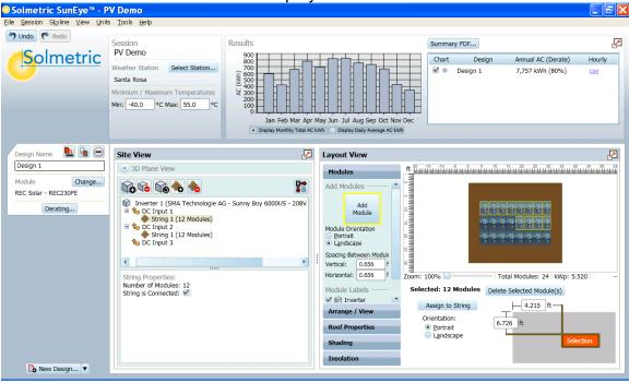
Note: Limit checks are performed on the designs to ensure that the string voltage and power are within the specifications of the inverter. These values are very dependent on the minimum and maximum temperatures. To set the temperature minimum and maximum, enter them in the Weather Area to the left of the Results Area.
