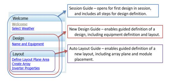
Note that these guides are used for simplified access to the features required for definition of the design and layout. As an alternative, designs and layouts can be entered in Manual Mode. Or initial preliminary designs can be created using the Guides, and then modified in Manual Mode. With this combination, PV Designer enables the user to combine ease of use of the Guides with the flexibility of Manual Mode.
