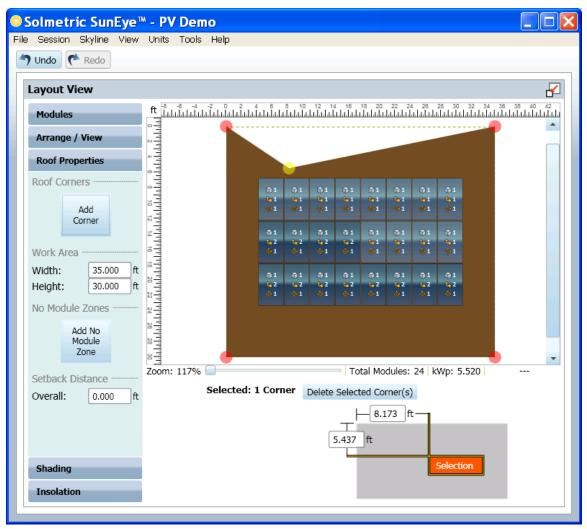
Repeat this process of adding and adjusting corners until the desire roof shape is completed. An example with three added corners (total of seven) is shown below.
