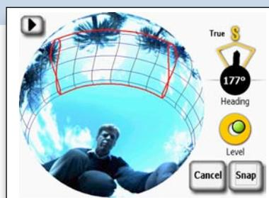
**Target mode** enables accurate measurements even when nearby metal distorts compass readings.
