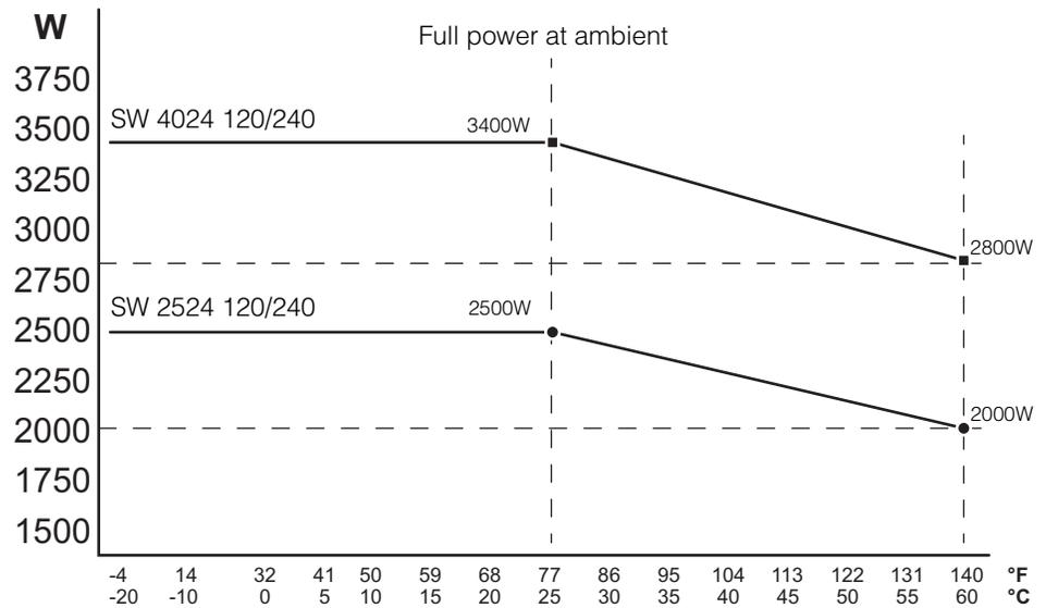
Figure 6-1 Output Power versus Temperature Derating Graph
