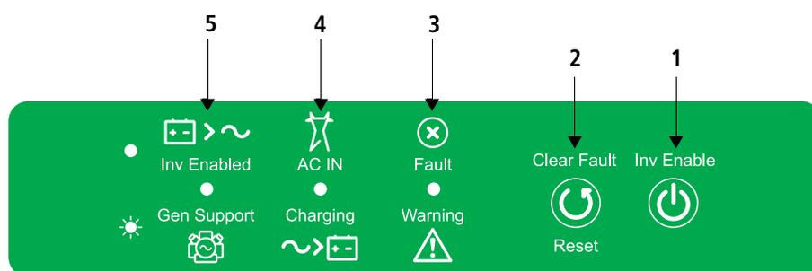
Figure 2-3 Front Panel Buttons and Status LEDs
