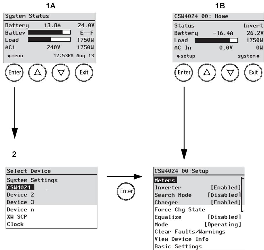
Figure 3-7 Navigate To Conext SW Setup Menu
