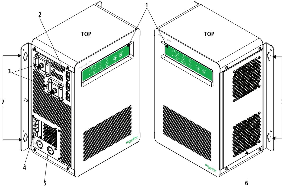
**Figure 2-2** Conext SW Front and Side Panels
