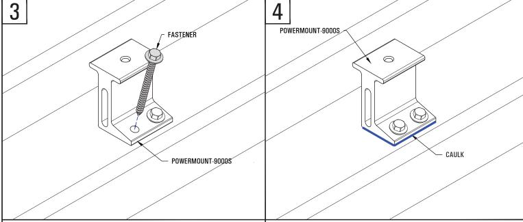
SECURE THE POWERMOUNT BY SCREWING THE SELF-TAPPING STAINLESS STEEL FASTENERS (INCLUDED) INTO/THROUGH THE PRE-PUNCHED HOLES, INTO/THROUGH THE EPDM GASKET, INTO/THROUGH THE ROOF PANEL, AND INTO/THROUGH THE ROOF DECK (IF APPLICABLE). MAKE SURE TO NOT OVER-TIGHTEN AS YOU RISK STRIPPING THE FASTENER. IF A FASTENER IS STRIPPED, REMOVE AND REPLACE WITH A SIMILAR FASTENER, BUT OF A LARGER DIAMETER.
