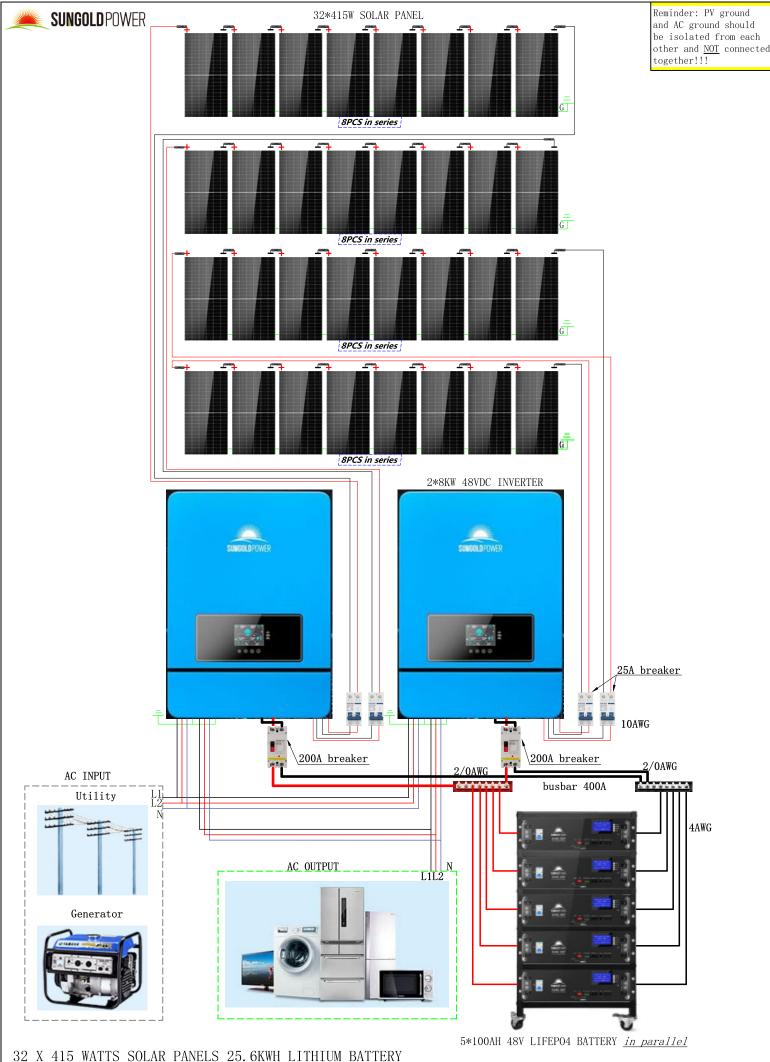
32 X 415 WATTS SOLAR PANELS 25.6KWH LITHIUM BATTERY 16KW SOLAR INVERTER 48VDC 120V/240VAC
