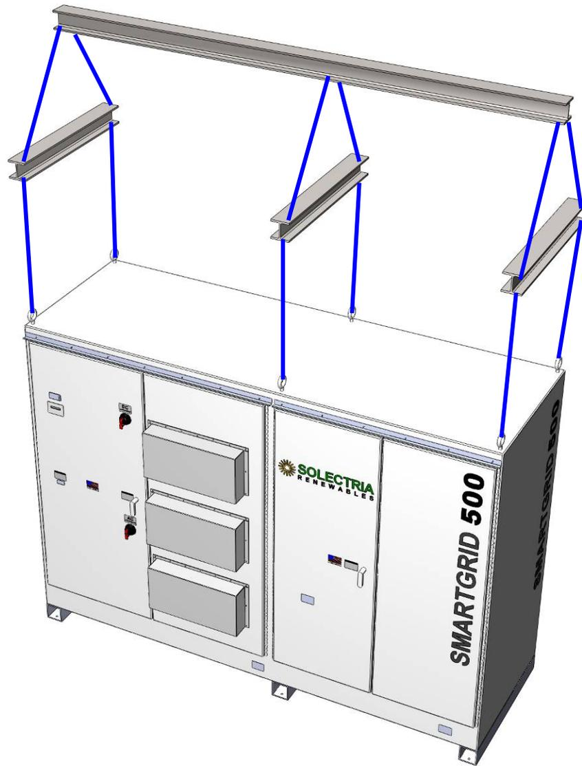
**Figure 3.2 – Preferred Straight-Chain Lifting Method**
