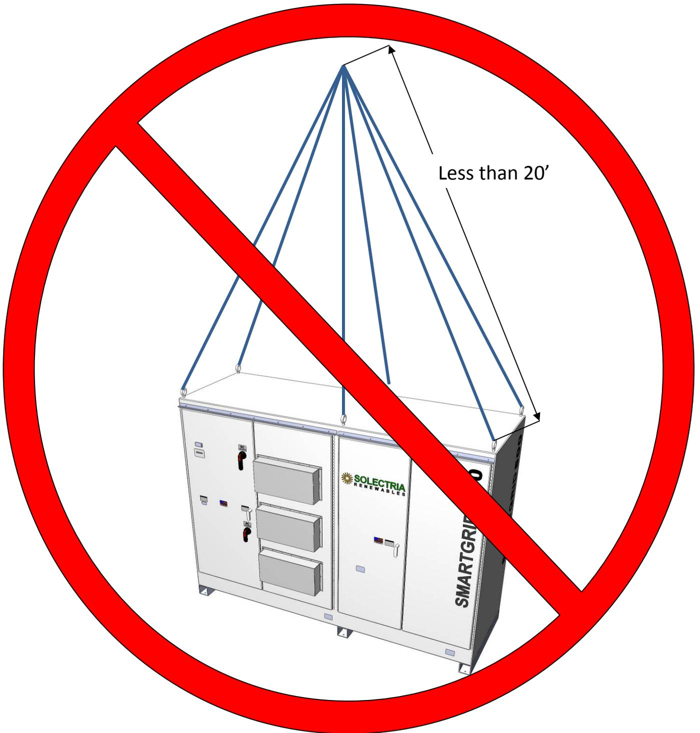
**Figure 3.5 – Improper Lifting Method**
