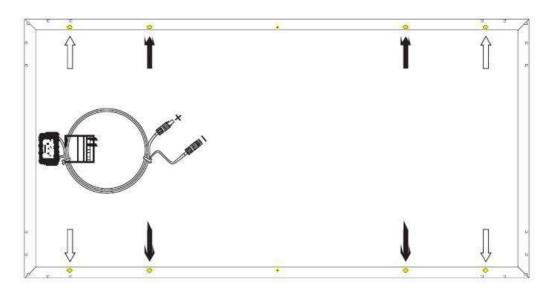
**†** Mounting holes for normal installation
