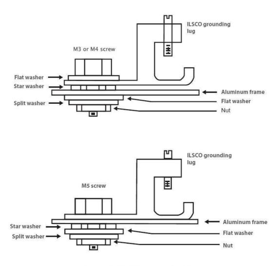
For module with Φ5.1mm grounding holes
