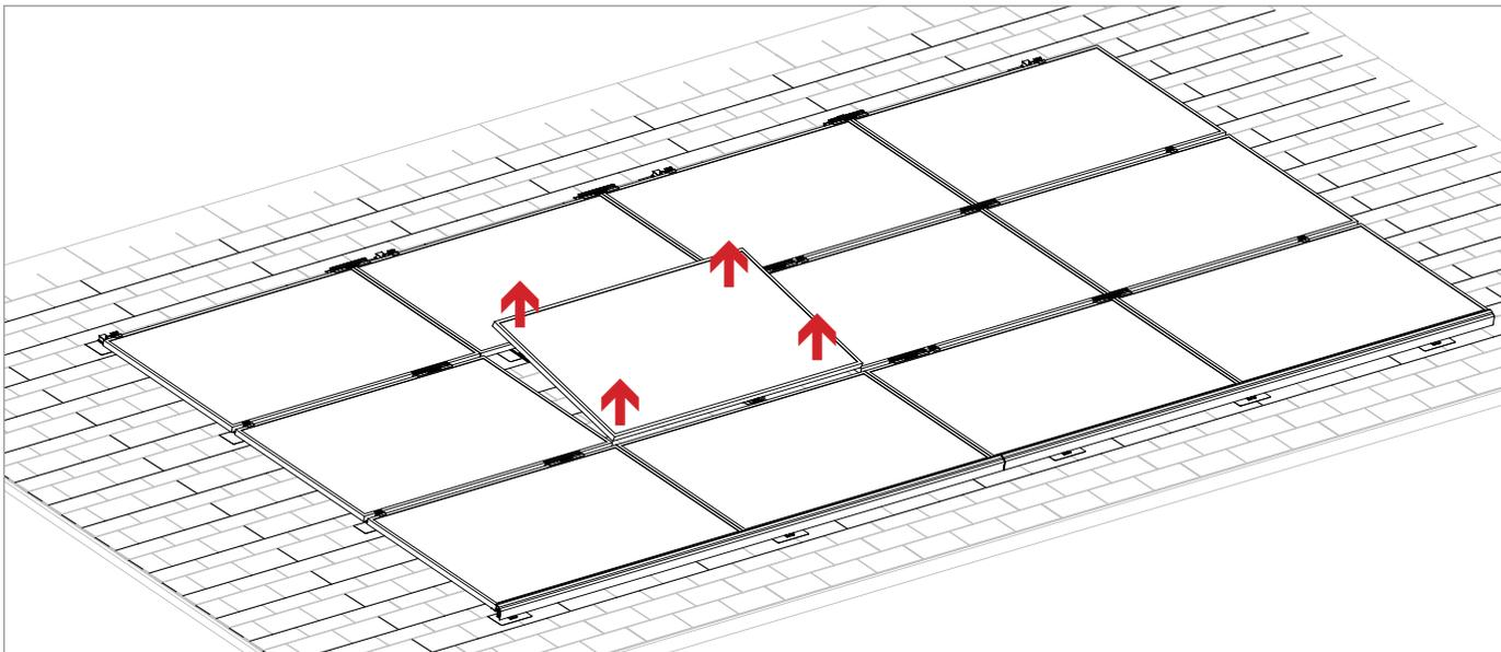
**REMOVE MODULE. REVERSE STEPS TO REPLACE MODULE REMOVED**
