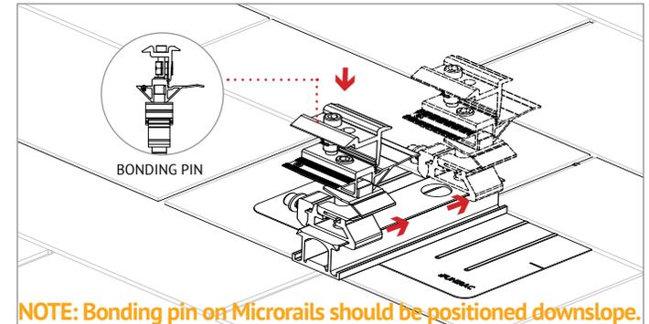
**NOTE:** Bonding pin on Microrails should be positioned downslope.
