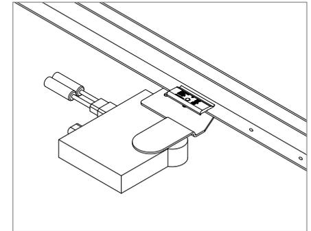
**LIFT MODULE AND DISCONNECT MLPE CABLES**
