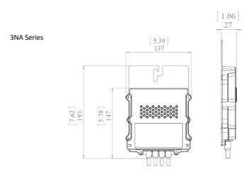
Figure 40: Power Optimizer Dimensions - mm/[inch]
