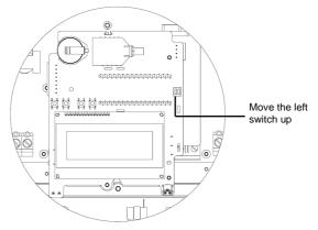
Figure 32: RS485 termination switch
