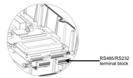
Figure 29: The RS485/RS232 terminal block
