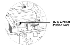
Figure 28: The RJ45 Ethernet connector
