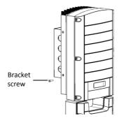
Figure 16: Inserting the screws into the outer heat sink fins
