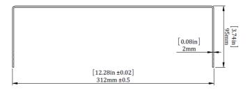
Figure 39: Three phase inverter mounting bracket
