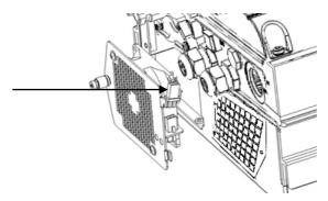
Figure 43: Fan connector
