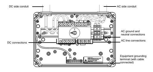
Figure 18: Inside the AC/DC Safety Switch for three phase inverters (DCD-3PH-US-S3-A)
