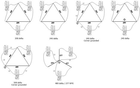
Figure 2: AC grids supported by SolarEdge single phase inverters
