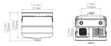
Figure 38: Three phase inverter with brackets - top and bottom views
