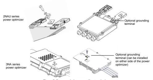
Figure 5: Power optimizer grounding terminal
