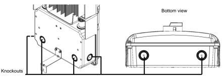
Figure 12: AC/DC Safety Switch knockouts
