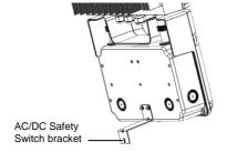
Figure 15: AC/DC Safety Switch bracket
