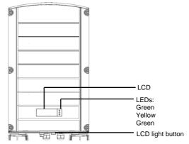
Figure 10: Inverter front view
