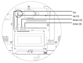
Figure 22: LCD internal user buttons
