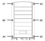
Figure 33: Tightening Order of the Screws
