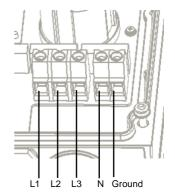
Figure 48: Three phase inverter AC terminals
