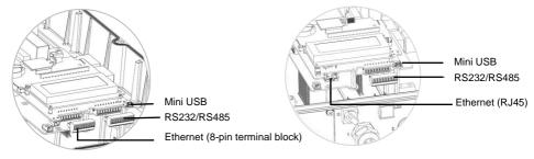
Figure 24: Internal connectors
