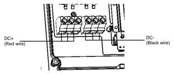
Figure 46: Three phase inverter DC terminals
