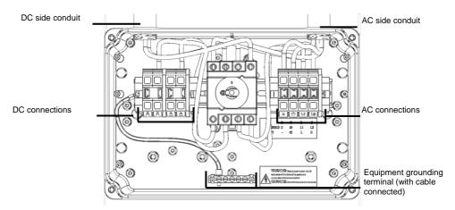
Figure 17: Inside the AC/DC Safety Switch for single phase inverters (DCD-1PH-US-C)
