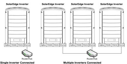
Figure 25: Example of Ethernet connection
