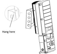
Figure 14: Hanging the inverter on the bracket
