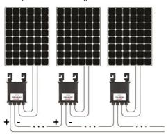
Figure 7: Power optimizers connected in series
