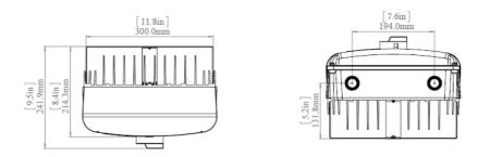
Figure 35: Single phase inverter with brackets - top and bottom views
