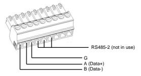
Figure 30: RS485/RS232 terminal block
