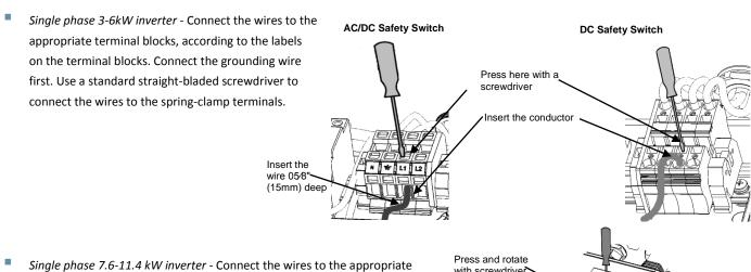
Single phase 7.6-11.4 kW inverter - Connect the wires to the appropriate terminal blocks, according to the label on the terminal blocks. Connect the grounding wire first. Use a 03/16" (5mm) straight flat-blade screwdriver to connect the wires to the terminals.
