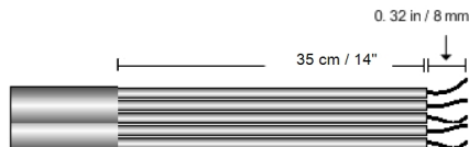
Figure 33: Insulation stripping – AC
