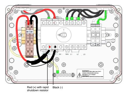
Figure 2: Three-phase inverter Safety Switch - connecting the Rapid Shutdown cable
