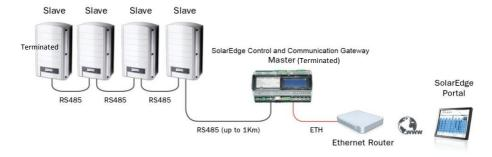
Figure 5: Example of RS485 Connection
