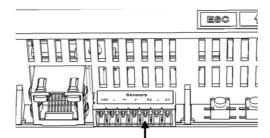
Figure 16: Sensor Interface Inputs
