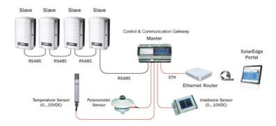
Figure 14: Example of Sensor Connection to the SolarEdge Gateway
