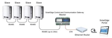
Figure 6: Example of Ethernet Connection
