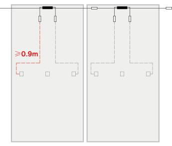
NOTE: The output cable length of integrated junction box PV module should be no less than 0.9m.
