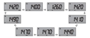
Press the **SET UP button** again, the selected battery type will be solidly On and confirmed.
