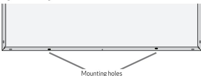
Fig. 6: Mounting using mounting holes
