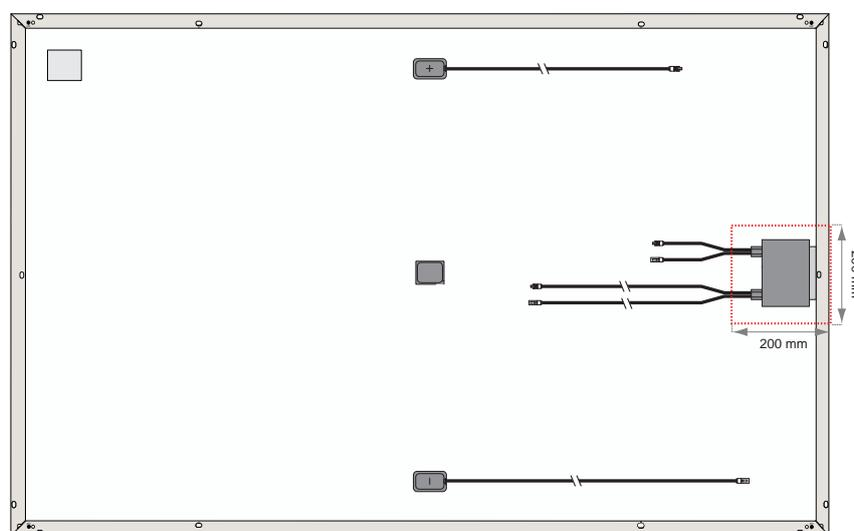
**⚠ Ensure that no rails are installed in the Rail Exclusion Zone around the power optimizer as this may interfere with or damage the power optimizer unit. The Rail Exclusion Zone measures 200 mm x 200 mm as marked in red in the above diagram.**
