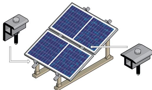
**⚠ In areas of snow build-up panels can be subjected to forces in excess of the stated limit even when snow depth does not appear extreme, causing damage to the framework. If the installation is likely to be affected by this, further suitable panel support is recommended on the lower row of panels.**
