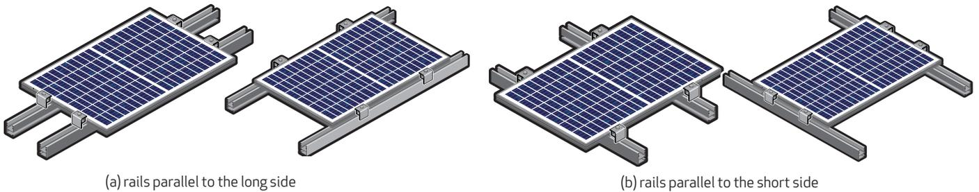
**★ The overlap between the support rail and the outer edge of the frame must be a minimum of 6 mm.**
