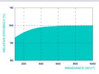
Typical module performance under low irradiance conditions in comparison to STC conditions ( $25\,^{\circ}$ C,  $1000\,\text{W/m}^2$ ).
