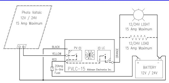
The PVLC-15 charges the battery from the solar PV panel during the day. At dusk the PVLC-15 senses the low PV panel voltage and turns on the light for the selected time period. The light will automatically turn off at dawn. In the Sign option, the PVLC-15 also turns on the light two hours before dawn.
