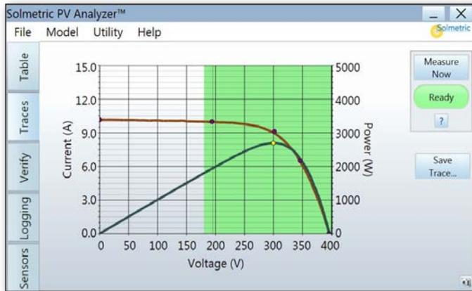
I-V and P-V curves of a healthy PV string. Inverter MPPT voltage range is highlighted in green.
