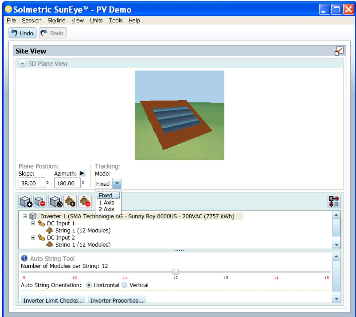
The 3D Site View can be collapsed to enable more optimal viewing of the Design Tree and properties of inverters and strings that are selected.
