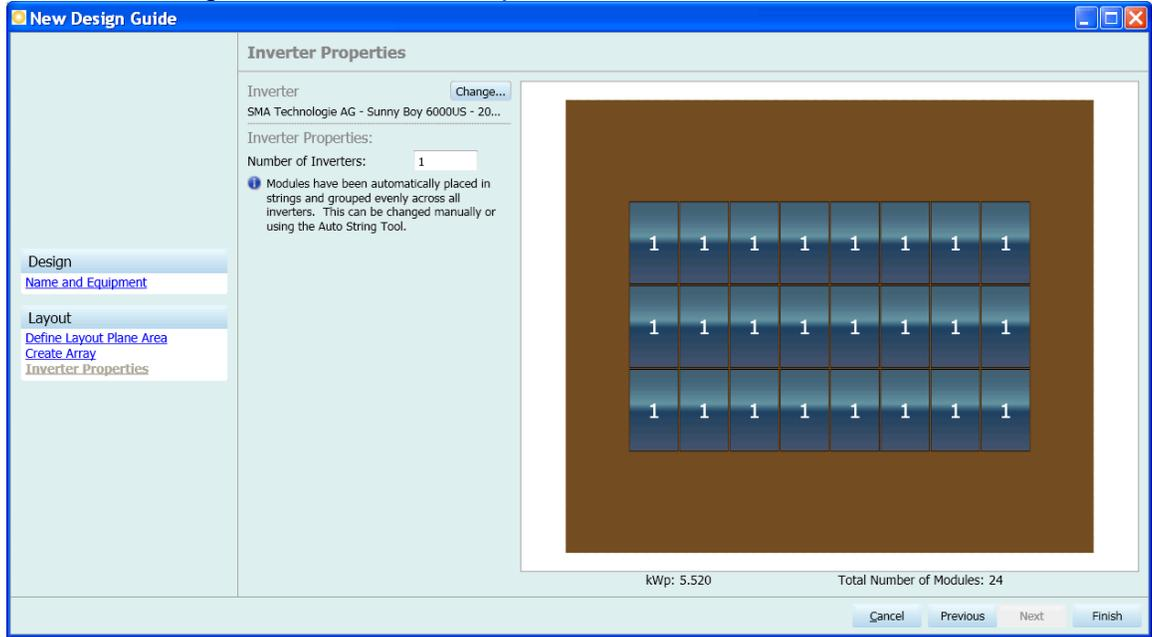
Enter or change the Inverter manufacturer and model, and the number of inverters. Note that the number of inverters must be between one and the number of modules. For microinverters, the number of inverters should equal the number of modules.
