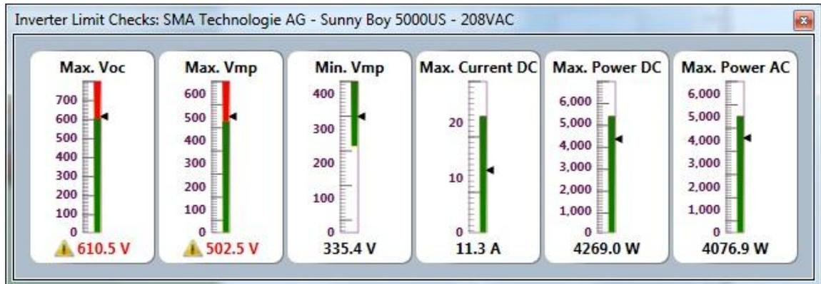
Green bars only are shown when the limits are not exceeded, and the arrow on the right of each value shows the calculated value. If limits are exceeded, a red bar is shown in addition to the yellow caution triangle, as shown above for DC Power and AC Power.
