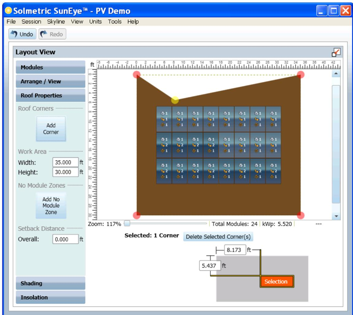
Repeat this process of adding and adjusting corners until the desired roof shape is completed. An example with three added corners (total of seven) is shown below.
