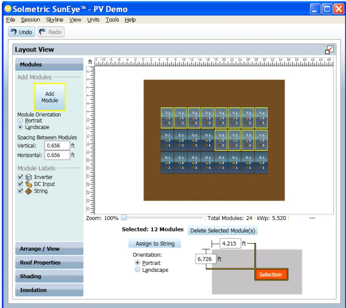
When a module or combination of modules is selected, the location is specified in the Properties Area. The position of the upper left corner of the selection is displayed, relative to the upper left corner of the array plane. For example, in the diagram below, the upper left corner of the selected modules is 4.215 feet over and 6.726 feet down from the upper left corner of the array plane.
