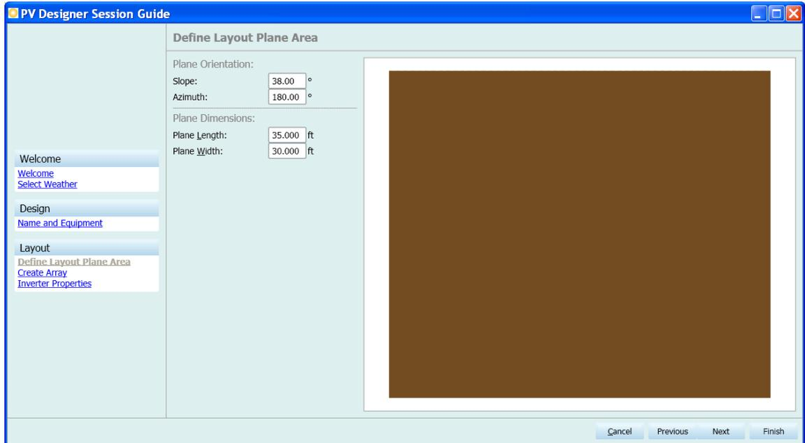
Set the Plane azimuth and slope, then the plane dimensions.
