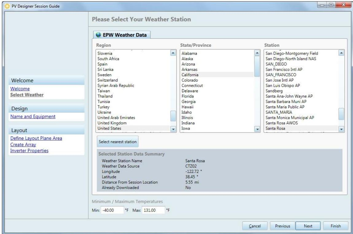
Note that the PV Designer Weather Station may be different from the Weather Model used for the Solmetric SunEye and the Solmetric SunEye Desktop Companion. The weather station selection in the PV Designer software is independent of the selection in the SunEye software. The weather station data must be reselected when using the session data in PV Designer Software.
