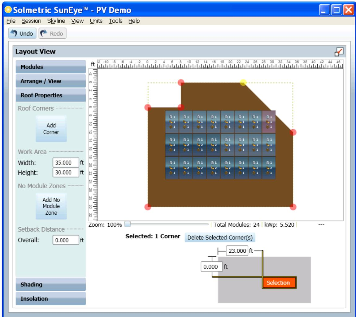
Note that one module is now outside the roof area, and is highlighted so that the user can be alerted to make adjustments.
