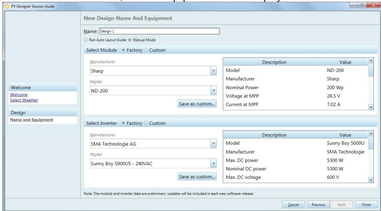
Select the manufacturer, then the model number from the drop down menus. The specifications available from the database are then shown in the display area. The default is for a “Factory” equipment with pre-stored specifications. “Custom” equipment can also be defined as described below.
