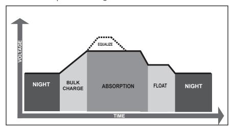
Figure 4.2. ProStar MPPT Charging Algorithm
