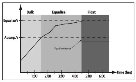
Figure 4.6. Equalize Time-out Charging Profile
