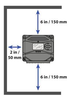
Figure 3-2. Proper Clearances for Passive Cooling
