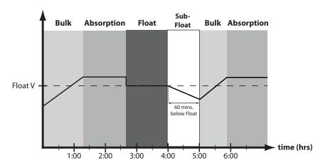
Figure 4-4. Float Exit Time-out Charging Profile
