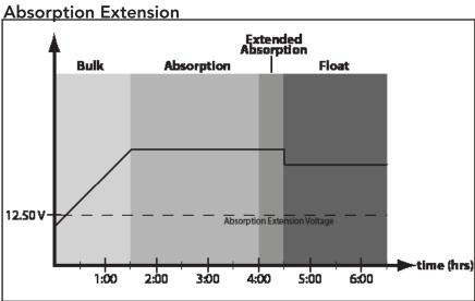
Figure 4-3. Absorption Extension Charging Profile
