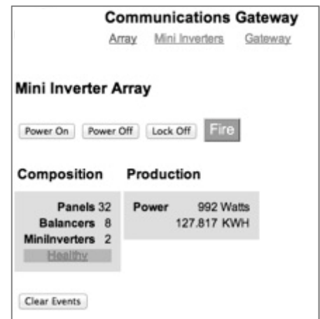
Figure 28: Web interface for the Gateway showing array statistics
