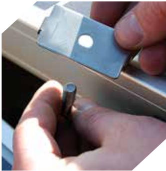
Lock-In-Place RAD Bolt
