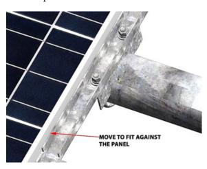
Loosen the End Clamp U-Bolts if necessary and move it to fit firmly against the solar module frame and retighten to hold position.
