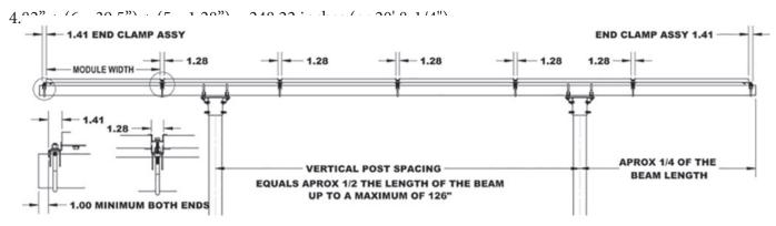
When using a single vertical pole (4" Sch-40 pipe) (1-4 modules) center the beam over the vertical post.
