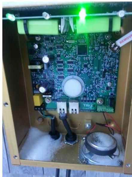
The PCB area of that same Birdhouse. The fine powdery snow had no trouble finding its way in through the unsealed edges. Some of the mounting holes were left unused providing more access to insects and the elements. The battery insulator tab was not removed either.
