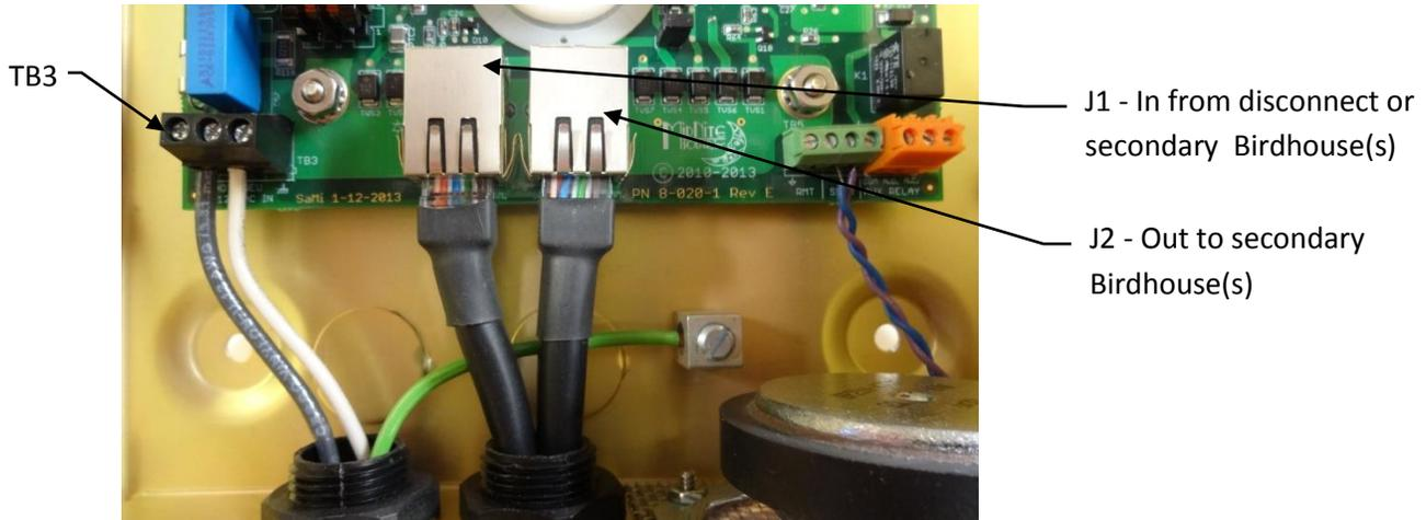
7. Connect the 600 volt UV rated CAT-5 control cable to the disconnect at J1. Use a small amount of silicone grease on all cable ends to protect the connections and repel moisture.
