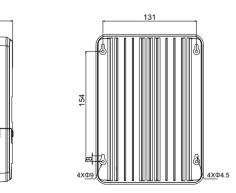
**RS-MPPT20** Product dimensions: 210\*151\*59.5mm Hole positions: 154\*131mm Hole diameter: Φ3mm Applicable wire: max. 8 AWG
