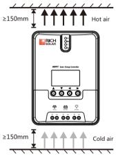
Fig. 2.1 Installation and heat dissipation
