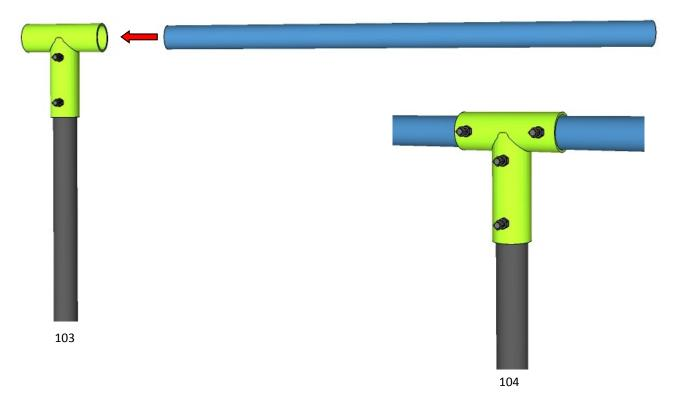
103: Slide the 2" Pipe into the Pole Cap Sleeve.
