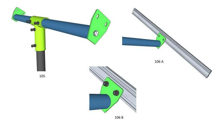
105: Attach the Rail Adapters to the ends of the 2" Pipe and tighten.
