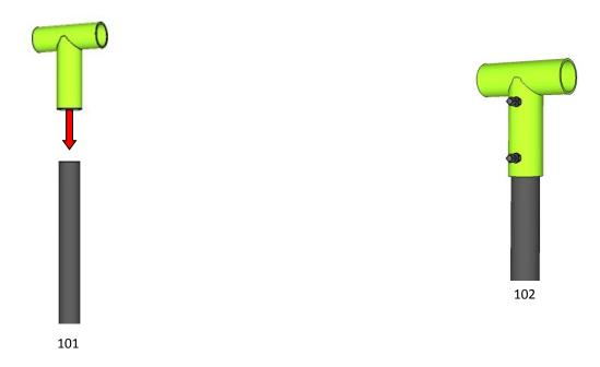
101: With the 2" Sch 40 pipe installed in the ground, slide the pole cap over the pipe.
