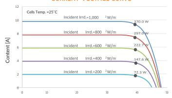
Voltage [V] Current-voltage characteristics with dependence on irradiance and module temperature
