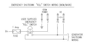
A double pole "kill switch" wired and installed by the user, stops the generator instantly in emergency situations such as a fuel spill. One switch pole (N.C.) kills power to the GSCM-mini-D opening all relays. The other switch pole (N.O.) shorts out the magneto for an instant stop.
