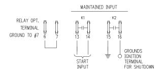
The K1 relay provides a continuous run signal for generators requiring a "maintained" start signal. The K2 relay provides a momentary "stop" signal until the generator AC Hz has dropped to zero. For GSCM-mini-D operational sequence details see Page 4, Section - 2
