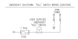
A single pole "kill switch" wired and installed by the user, stops the generator instantly in emergency situations such as a fuel spill. One switch pole (N.C.) kills power to the GSCM-mini-D opening all relays shutting down the ignition switch type generators.
