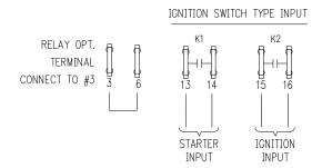
The K1 relay is used to switch the starter input that is looking for a momentary signal and opens it when the AC line output has reached 45Hz. The K2 relay provides a continuous run signal for generators requiring a "maintained" ignition signal. When the GSCM-mini-D no longer receives a run command, K2 relay opens telling the generator to shutdown. For GSCMmini-D operational sequence details see Page 5, Section - 3
