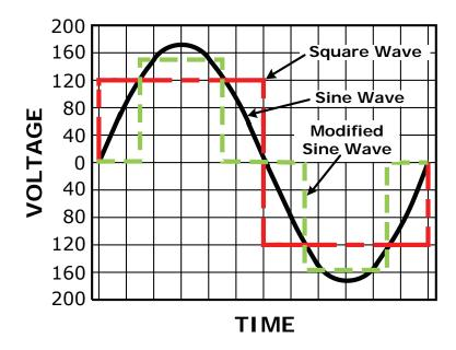
Figure 1-5, AC Waveforms
