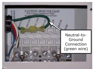
Figure 2-22, Disconnecting the Neutral-to-Ground Connection
