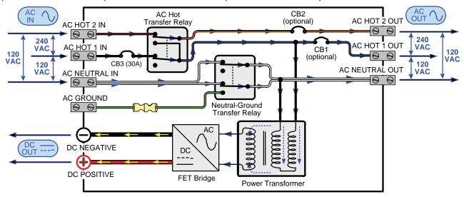
Figure 3-2, Power Flow - Standby Mode
