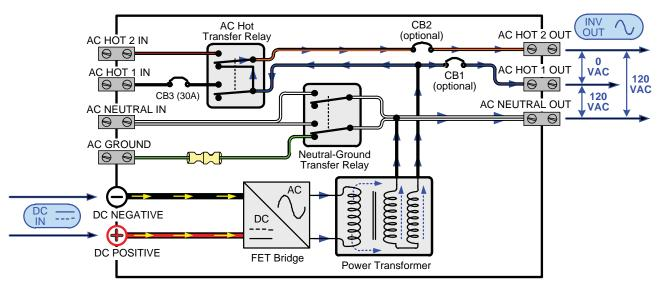
Figure 3-1, Power Flow - Inverter Mode
