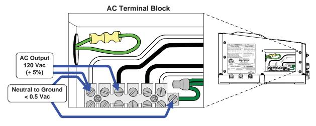
Figure 2-25, AC Voltage Checks
