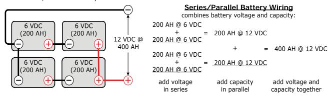
Figure B-3, Series-Parallel Battery Wiring
