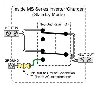
Figure 2-21, Neutral-to-Ground Connection (Standby Mode)
