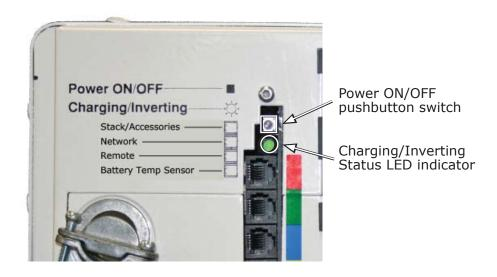
Figure 3-5, Power Switch and Status Indicator
