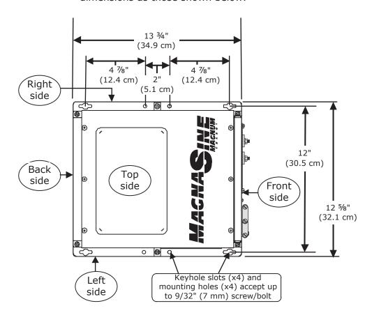
Figure 2-3, MS Series Dimensions and Side Reference
