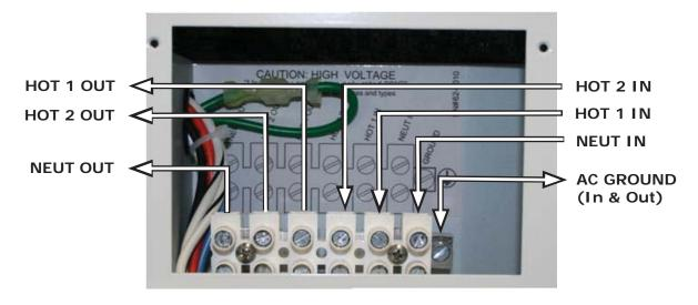
Figure 2-8, AC Terminal Block
