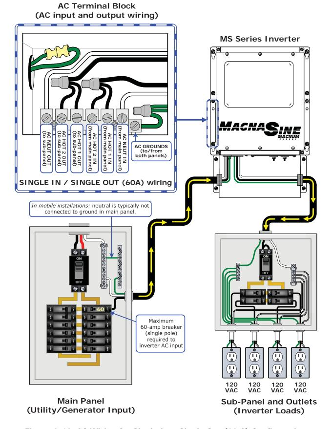
Figure 2-10, AC Wiring for Single In – Single Out (60 A) Configurations
