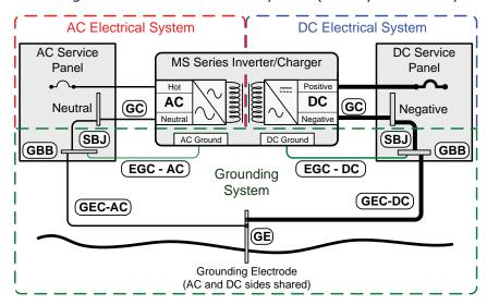
Figure 2-18, Multiple Connections to DC Ground Rod (Method 2)
