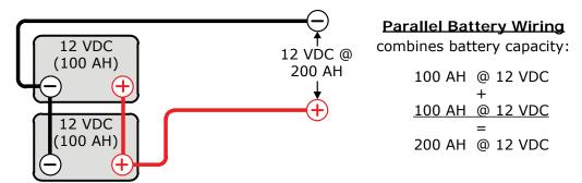
Figure B-2, Parallel Battery Wiring
