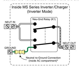
Figure 2-20, Neutral-to-Ground Connection (Inverter Mode)
