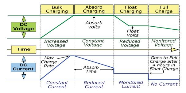
Figure 3-3, Automatic 4-Stage Charging Graph
