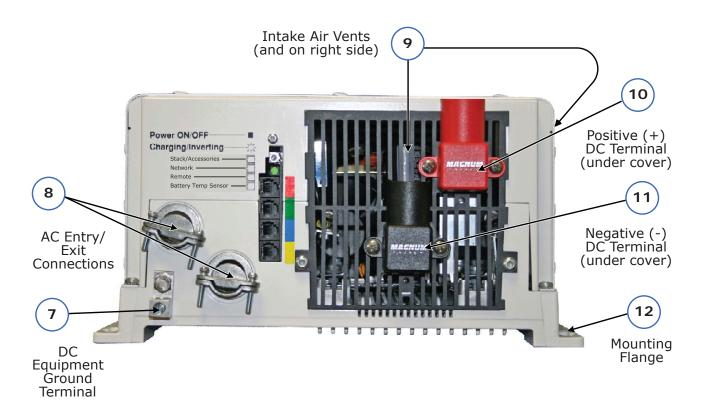
Figure 1-2, Electrical Connection Points
