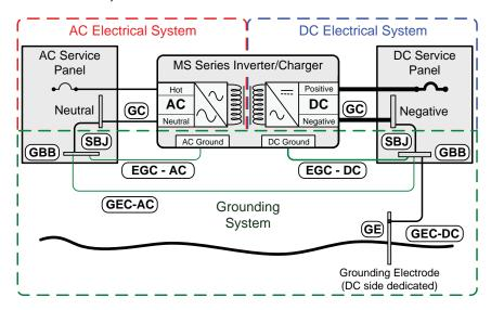
Figure 2-19, Single Connection to DC Ground Rod (Method 3)
