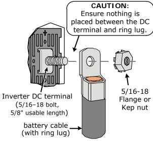
Figure 2-6, Inverter DC Hardware Installation
