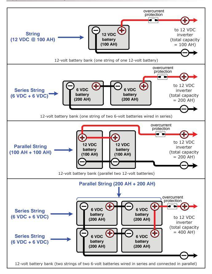
Figure B-4, Battery Bank Wiring Examples (12-volt)
