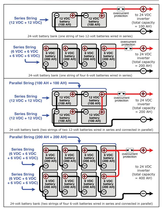
Figure B-5, Battery Bank Wiring Examples (24-volt)
