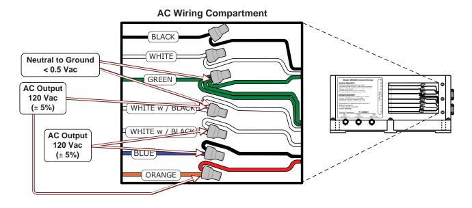
Figure 2-27, AC Voltage Checks (MS2000-15B/20B models)
