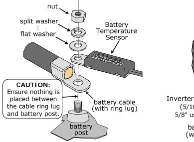
Figure 2-5, Battery Hardware Installation
