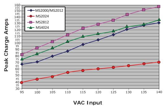
Figure A-2, MS Series VAC Input to Charge Amps
