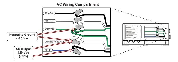
Figure 2-26, AC Voltage Checks (MS2000 models)
