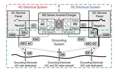
Figure 2-16, Grounding System for MS Series
