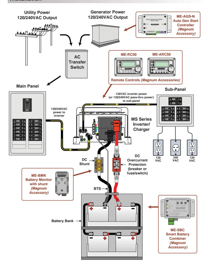
Figure 2-1, Simplified Installation Diagram for Permanent Installations
