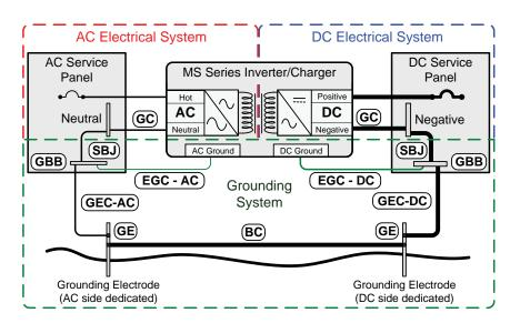
Figure 2-17, Multiple Connections to DC Ground Rod (Method 1)
