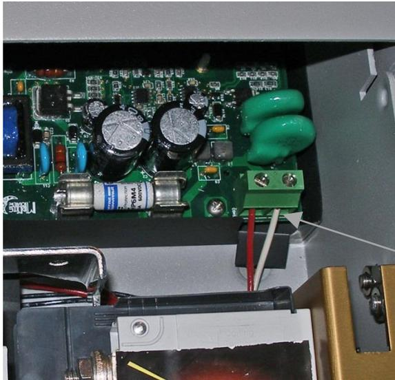
**Step 7:** Strip one end on the red and white wires included in the kit ¼" and connect them as shown with the red wire on the left side of the terminal block marked "PV+" and the white wire on the right side marked "PV-". Route the wires downward under the large switch.
