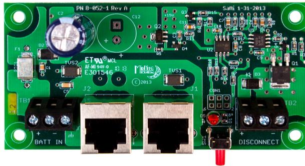
Accessory for use with most MidNite Disconnecting combiners as part of a Rapid System Shutdown.
