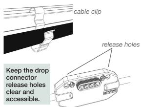
**b.** Dress any excess cabling in loops so that it does not contact the roof.
