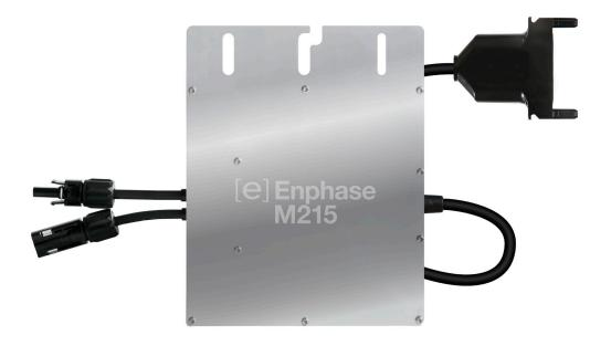
The **Enphase**<sup>®</sup> **M215 Microinverter** with integrated ground delivers increased energy harvest and reduces design and installation complexity with its all-AC approach. With the advanced M215, the DC circuit is isolated and insulated from ground, so **no Ground Electrode Conductor (GEC) is required for the microinverter.** This further simplifies installation, enhances safety, and saves on labor and materials costs.
