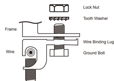
Figure 7: Installation Methods
