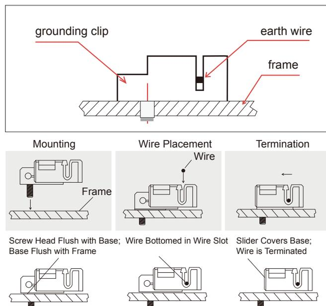
Figure 6: Installation Methods
