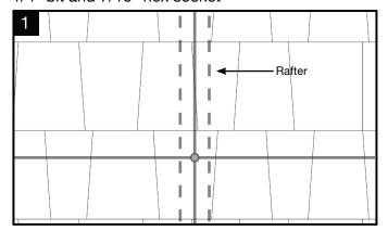
Locate rafters and snap vertical and horizontal lines to mark locations of flashings. Drill 1/4" pilot holes, then backfill with roofing manufacturer's approved sealant.
