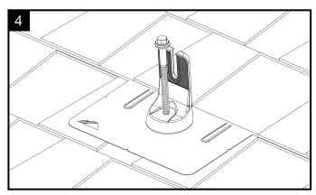
Insert Lag Bolt through Cap and flashing. Tighten lag bolt until fully seated. FlashVue with GripCap+® is now installed and ready for IronRidge® XR Rails®.
