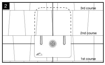
Slide flashing between 1st and 2nd course, so the top is at least 3/4" above the edge of the 3rd course and the bottom is above the edge of the 1st course. Line up pilot hole with flashing hole.
