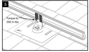
Attach rails to either side of the open slot using bonding hardware. Level rail at desired height, then torque to 250 in-lbs (21 ft-lbs).
