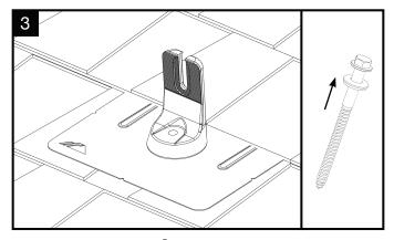
When installing Gripcap+® on roofs with undulations greater than 1 inch, install GripCap+® in low points across the array as required. If removing a GripCap® to replace with GripCap+®, it may be required to loosen an already installed adjacent GripCap®. Be sure to replace washer with new provided washer and refill pilot hole with sealant.
